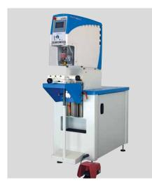
HERMETIC 60 with universal base frame, angle table, cross support and foot switch
