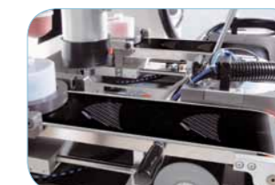
Integrated laser unit for production of printing clichés
